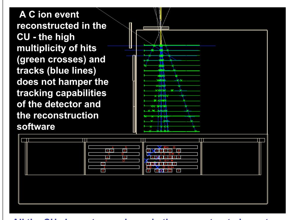
All the CU elements are shown in the reconstructed event: one TKR tower, 2 CAL modules and the top ACD tile are hit by ions while 4 ACD tiles and a complete TKR+CAL tower are not activated; the external container is also visible
