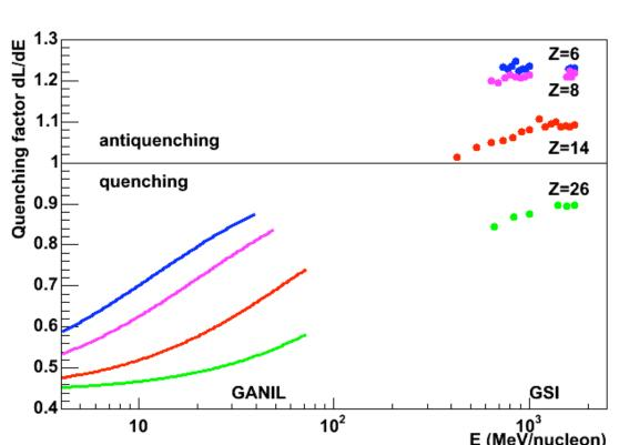
• QF measured on CsI in previous heavy ion beam test on a prototype of the GLAST CAL (NIMA 560-2006). A lower response wrt to a MIP was measured at low ion energy at GANIL, while an anti-quenching effect was recorded at high energy at GSI
