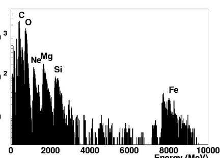
Expected distribution of ionization energy deposited by CR ions in one Csl crystal of the LAT CAL
