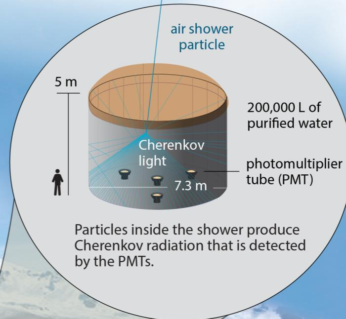
Particles inside the shower produce Cherenkov radiation that is detected by the PMTs.
