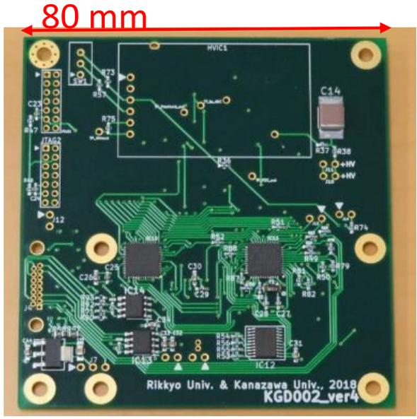
Prototype Readout Board
