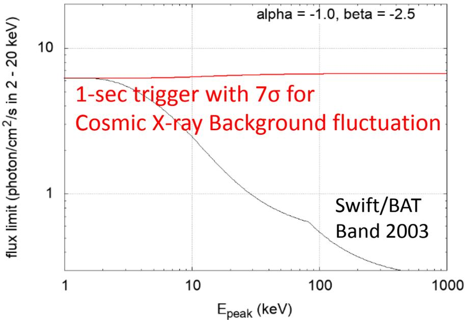
T-LEX has a comparable sensitivity for GRBs with  $E_{\text{peak}}$  of a few keV to *Swift*/BAT, and will efficiently detect GRBs with photon indices of  $> 2$ .
