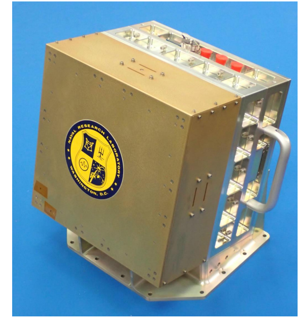
Fig. 3: Assembled TERI with dimensions 35(L) \times 35(W) \times 31(H) cm 3
