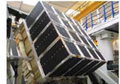
The LAT fully populated with TKRs (visible) and CALs, prior to installation of the ACD.
