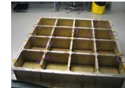
The 4x4 Grid provides mechanical support and thermal control for the detector array. CAL Modules are inserted into each bay, while TKR Modules mount to the upper edge of each bay.
