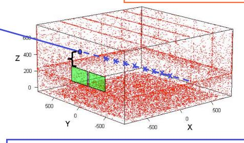
Because of backsplash, there may be struck tiles that are not associated with the tracks. Segmentation of the ACD allows us to salvage such events.
