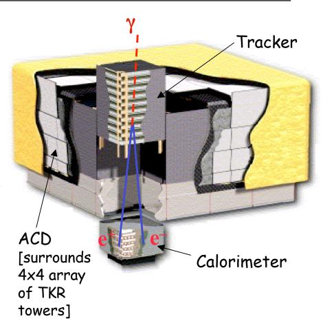
The systems work together to identify and measure the flux of cosmic gamma rays with energy ~20 MeV → ~300 GeV.
