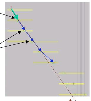
The search region is set by propagating the track errors through the LAT geometry.
