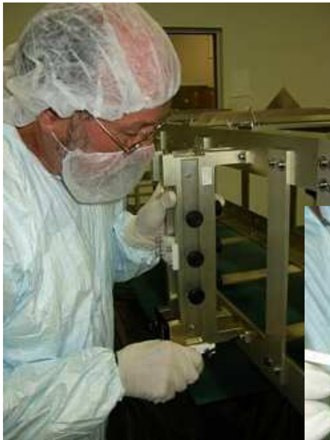
Hanging xtal in bonding fixture
